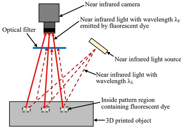
Figure 1. Basic concept of proposed technique [10]
