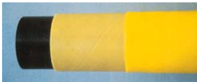
Figure 4. RTP pipe consists of a primary tube in HDPE (left), several crossed layers of Aramid yarns coated with HDPE (center), and an outer layer (right) of HDPE for external protection [13]
