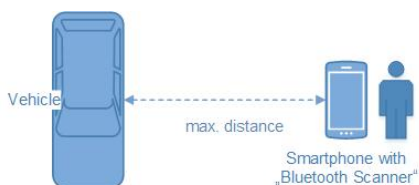
Figure 4. Test arrangement for the detection of Secondary Vehicle Identifier in stand still mode
