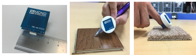
Figure 1. Overview of ZigBee microcomputer. Left: TWE-Lite-2525A [10]. ZigBee microcomputer: it includes a 3-axis accelerometer, a battery cell, and a communication module. Right: Overview of data collection.
