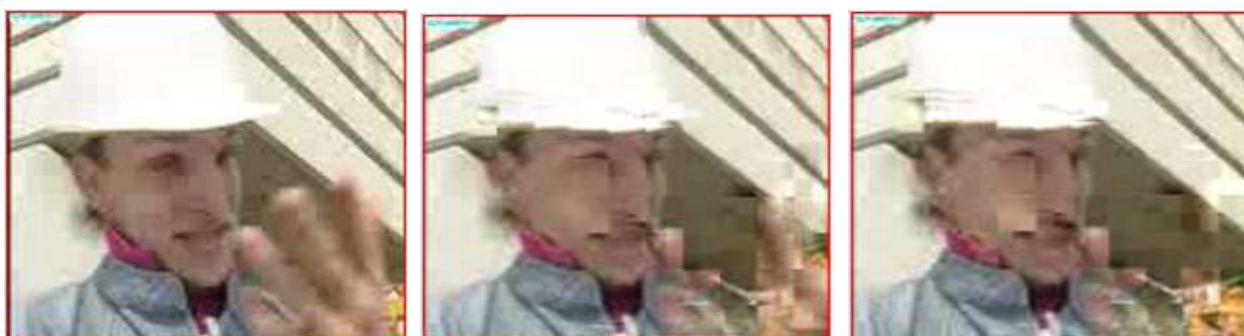
(b) Frames 156-158, PER @ 10% for GW encoded at 80kb/s
