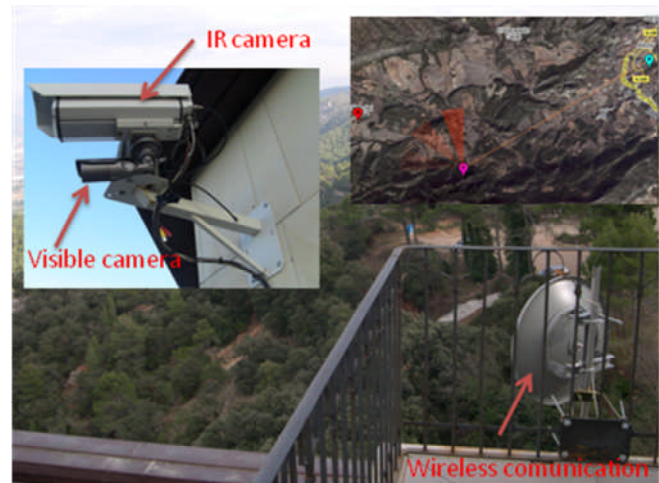
Figure 2. Real global system with infrared/visible cameras and wireless communication unit
