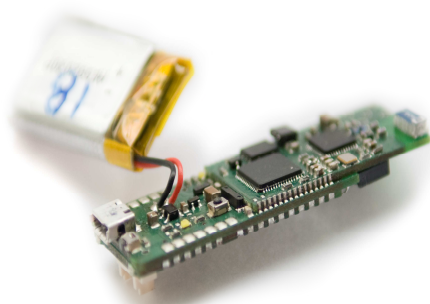
Figure 9. ASE-BAN node (processing and energy side).
