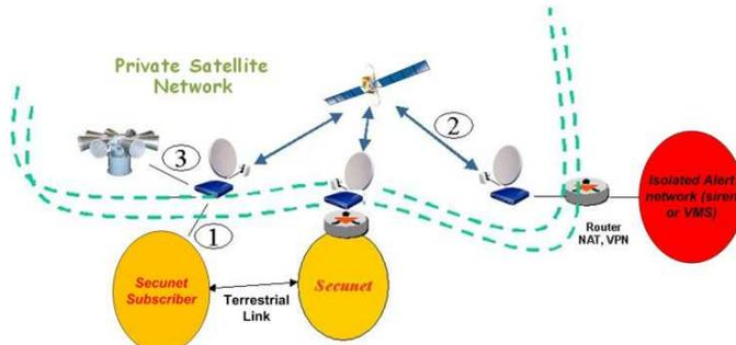
Figure 3. Ku Band Satellite Connection Systems
