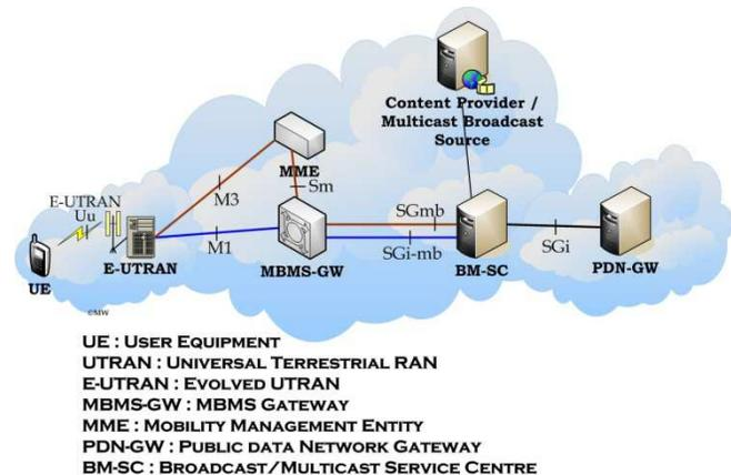
Figure 7. MBMS model in the LTE system
