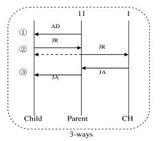
Figure 6. 3-ways handshake in MMT joining process
