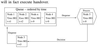
Figure 9. Example of scheduler instance in our discrete-event simulator.
