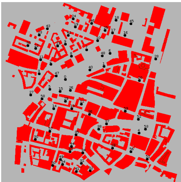
Figure 3. Simulation environment when number of nodes=60. Obstacles are printed red.
