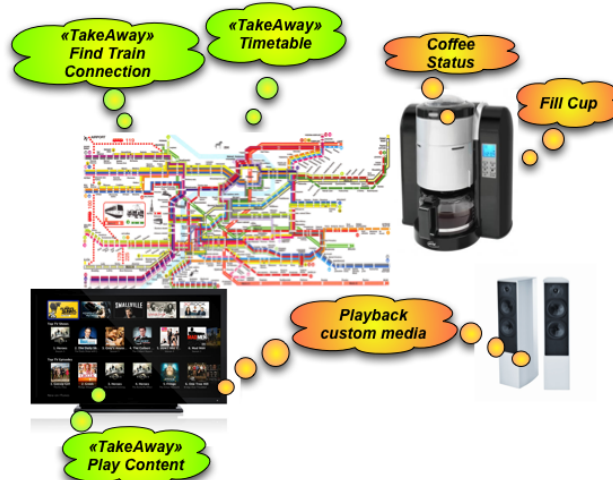
Figure 2. In this example, services with the takeaway-attribute are connected to a metro plan and a TV screens. The coffee-machine and speakers providing playback services but only allow direct interaction.
