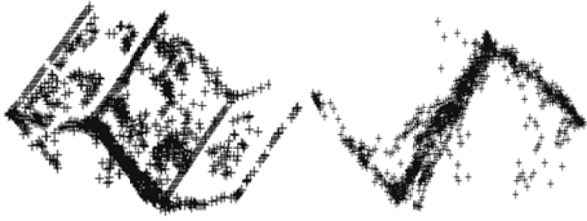
Figure 1. Wrong solution because perform 3D registration with two shapes in different groups.
