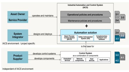
Figure 4. Application of IEC 62443 parts by different roles
