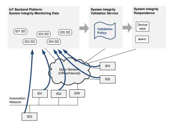
Figure 7. Validation of Device Monitoring Data
