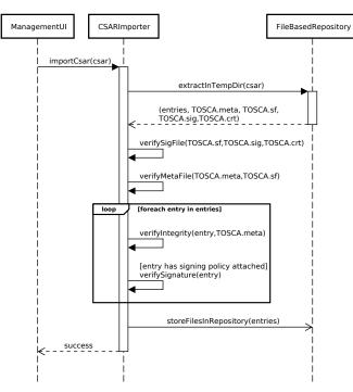
Figure 14. A simplified process of securely importing a CSAR showing only the successful control flow.
