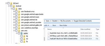
Figure 10. Wire cache and media files in Oxygen
