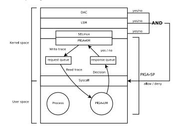
Fig. 6. Process to ensure the security properties at the Operating System layer
