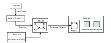
Fig. 4. Process of analyzing a SELinux policy and generating the patterns violating the security properties
