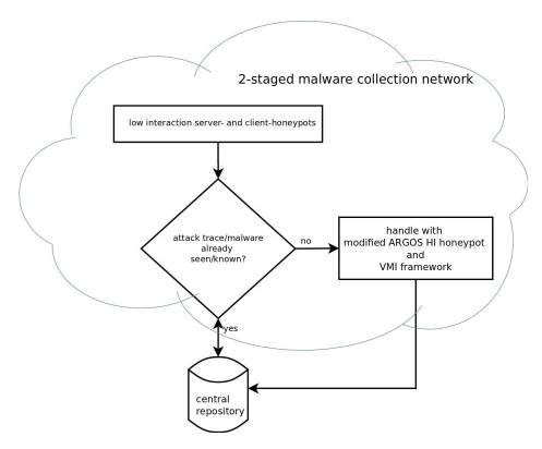
Figure 5. Scheme of the two-stage malware collection network.
