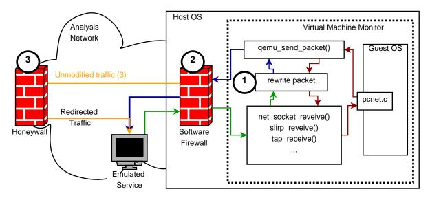
Figure 7. A connection could be redirected within virtual hardware, or the system call itself could be rewritten(1). The packets could be redirected using NAT, either by the virtualization host(2) or the honeywall(3).
