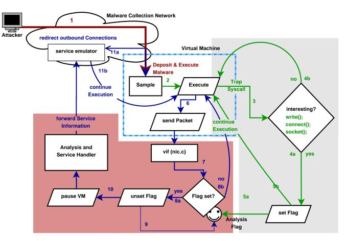
Figure 6. The gray area contains the system call tracing logic and will set a flag if a matching system call has been encountered. The red area holds the analysis components, which are activated only if the flag has been set.
