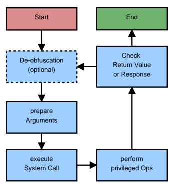
Figure 3. Privileged operations, such as network or disk operations, cannot be executed in user space. Software uses system calls to perform these operations in kernel space.
