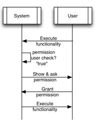
Figure 4. Sequence diagram: first use of one permission or a use or permission in 'user check' mode.
