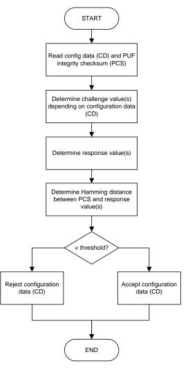
Figure 6. PUF-based Integrity Check of Configuration Data
