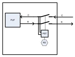
Figure 7. PUF Built-In Self Test
