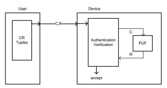
Figure 5. PUF Authentication Verification
