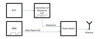
Figure 8. PUF-based Spread-spectrum Transmission
