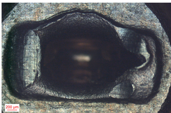
Figure 11. Image of mark after firing pin on cartridge case fired from Glock 17 measured with optical microscope.
