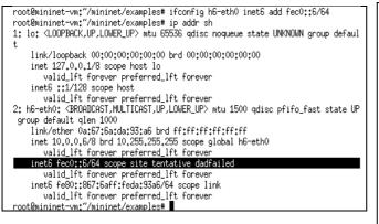
Figure 6. Screenshot of commands and output generated in h6 while testing non duplicate IPv6 address assignment with central arbiter module disabled on the controller and attacker active in h3
