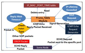
Figure 2. Pruning logic for the IP\_MAC\_PORT\_TIME table
