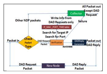
Figure 1. Workflow inside the Central Arbiter enabled SDN controller
