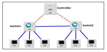
Figure 3. Topology of the test setup with 6 nodes
