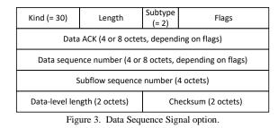
subflows, with sufficient control information to allow it to be reassembled and delivered to the receiver side application reliably and in order. The MPTCP connection maintains the *data sequence number* independent of the subflow level sequence numbers. The data and ACK segments may contain a *Data Sequence Signal (DSS)* option depicted in Figure 3.
