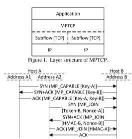
Figure 2. Example of MPTCP connection establishment.
