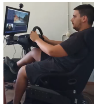
Figure 7. Driving simulation setup for integrating DMS and OFE.
