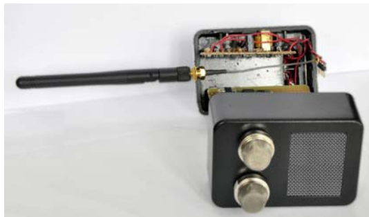
Figure 1. Wireless electronic node for environmental emergency application (e-nose). Here, it is possible to note the power supply modules with OFDM modem, the ZigBee transponder antenna and the gas sensors.
