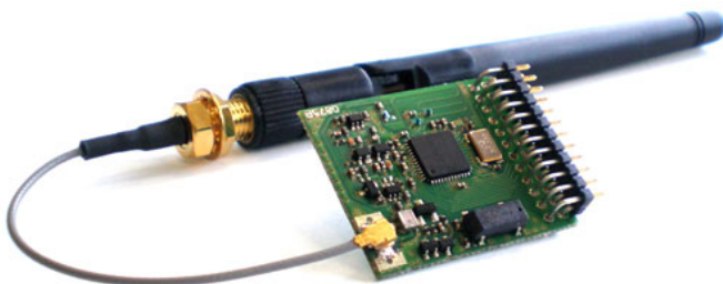
Figure 3. On the left: high power Aurel XTR-ZB1-xHE module, based on IEEE 802.15.4 standard and ZigBee protocol [15]; On the right: topology of ZigBee wireless networks: star, tree, and mesh.
