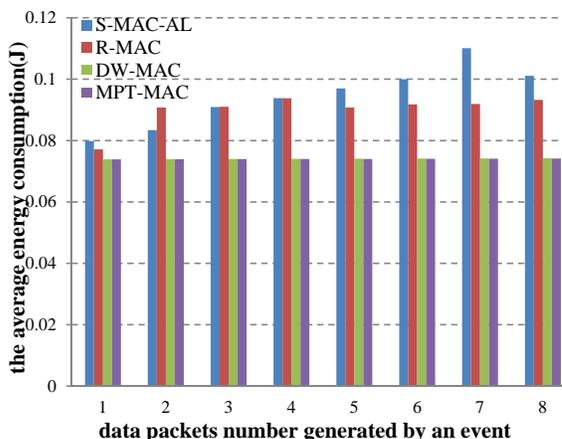
Fig. 13: Average energy consumption in the 7x7 grid network
