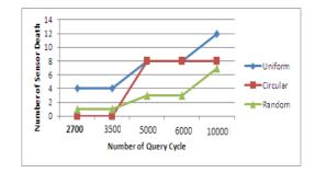
Figure 8. Rate of Sensor death for three Sensor Placement Strategies.
