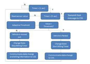
Figure 6. Flow Diagram at Sensor Mote
