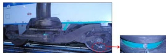
Figure 1. The temperature measuring on the axle box bearing
