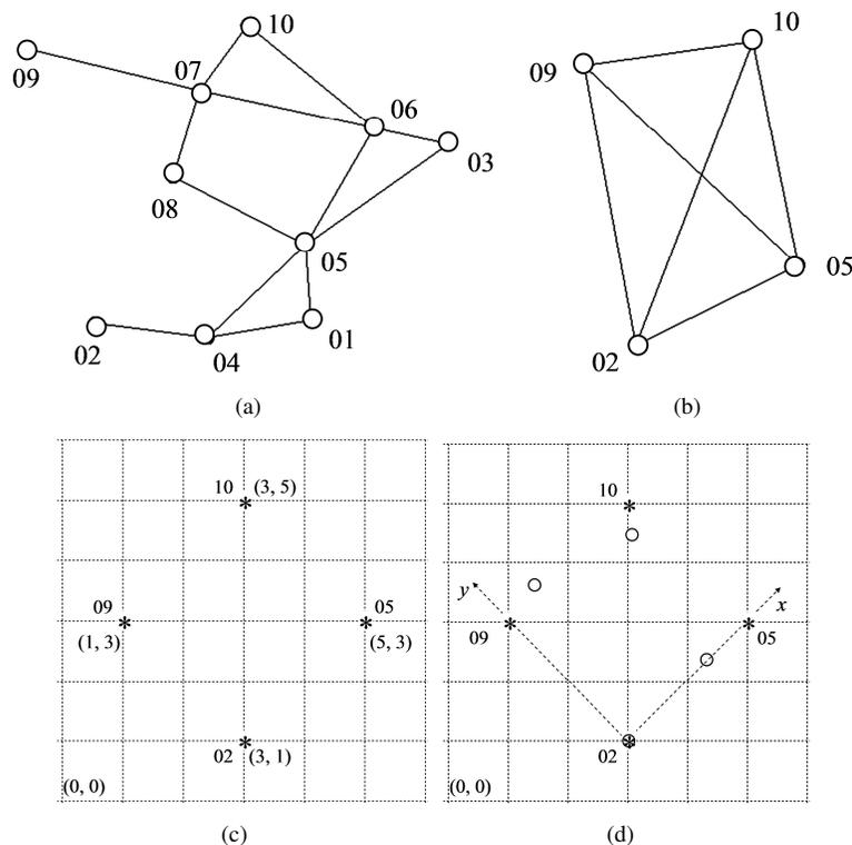
Fig. 1. Grid coordinate system establishment. (a) The constructed graph  $G(V, E)$  (b) The set of grid nodes for establishing the grid coordinate system. (c) The local grid coordinate system. (d) The transformed grid coordinate system.
