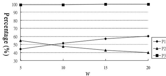
Fig. 6. The localization accuracy of non-grid nodes versus grid width.
