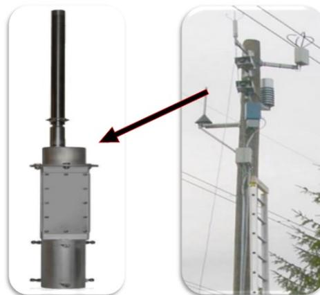
Figure 1. Ice Load Monitor [13]
