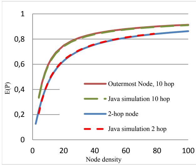
Figure 5. The expected value of the probability that dedicated recovery methods are not needed to mend routing path disconnections.
