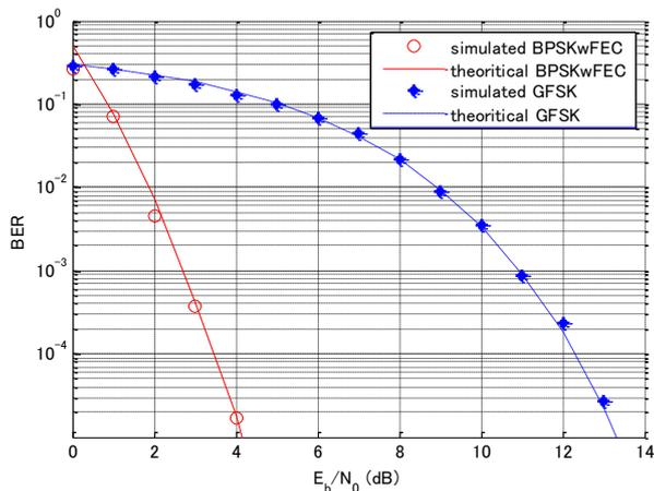
Fig. 4 BER performance comparison of 802.15.4k(BPSKwFEC) and 802.15.4g(GFSK) systems (theory and simulation)
