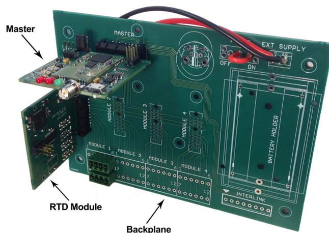
Figure 3. The MMS: master, RTD module, backplane
