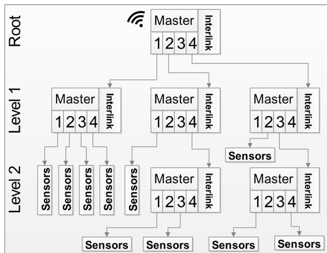
Figure 2. Interlink connections
