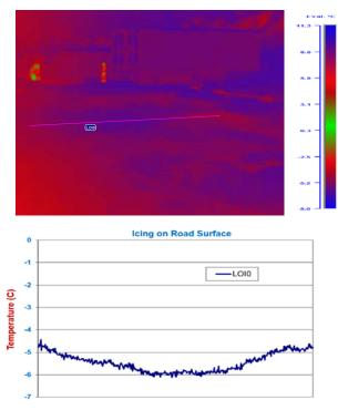
Figure 3. Surface temperature distribution along iced road surface.
