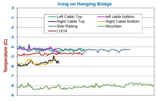
Figure 2. Surface temperature distribution along different sections of iced bridge
