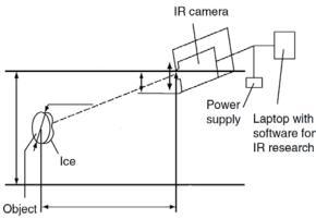
Figure 1. Schematic overview of field experimentation setup
