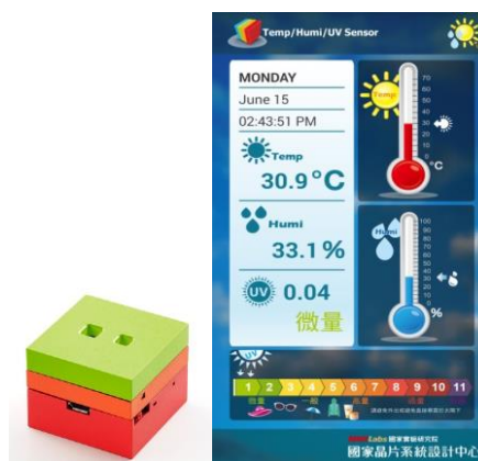
Figure 8 A temperature sensor system and its smart phone App.
