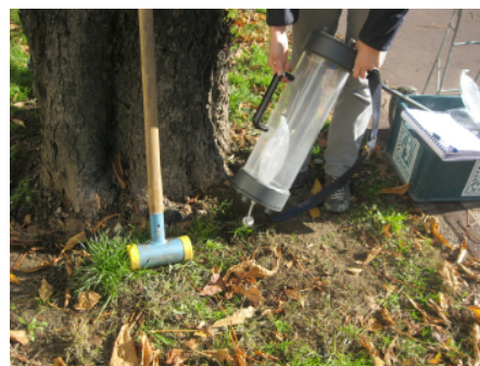
Figure 4. The automatic pump employed in the field to put directly soil air in Nalophan bags
