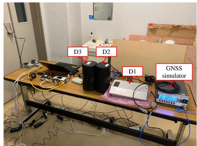
Figure 5. Indoor GNSS Time Information Delivery System.
