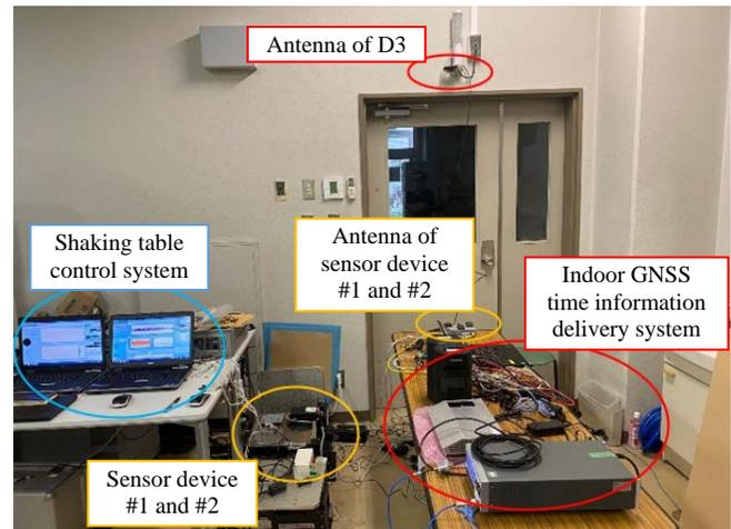
Figure 4. Overall View of Experimental System.
