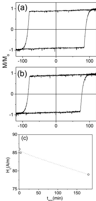
Figure 4. Hysteresis loops of as-prepared (a), and annealed at  $T_{ann} = 400$  °C for 180 min (b)  $Fe_{75}B_9Si_{12}C_4$  microwires and dependence of coercivity on annealing time (c).
