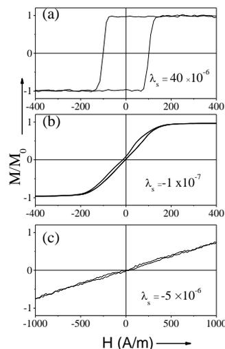
Figure 1. Hysteresis loops of magnetic microwires  $\text{Fe}_{75}\text{B}_9\text{Si}_{12}\text{C}_4$  with positive (a)  $\text{Co}_{67.1}\text{Fe}_{3.8}\text{Ni}_{1.4}\text{Si}_{14.5}\text{B}_{11.5}\text{Mo}_{1.7}$  with vanishing (b) and  $\text{Co}_{77.5}\text{Si}_{15}\text{B}_{7.5}$  with negative (c)  $\lambda_s$  values.
