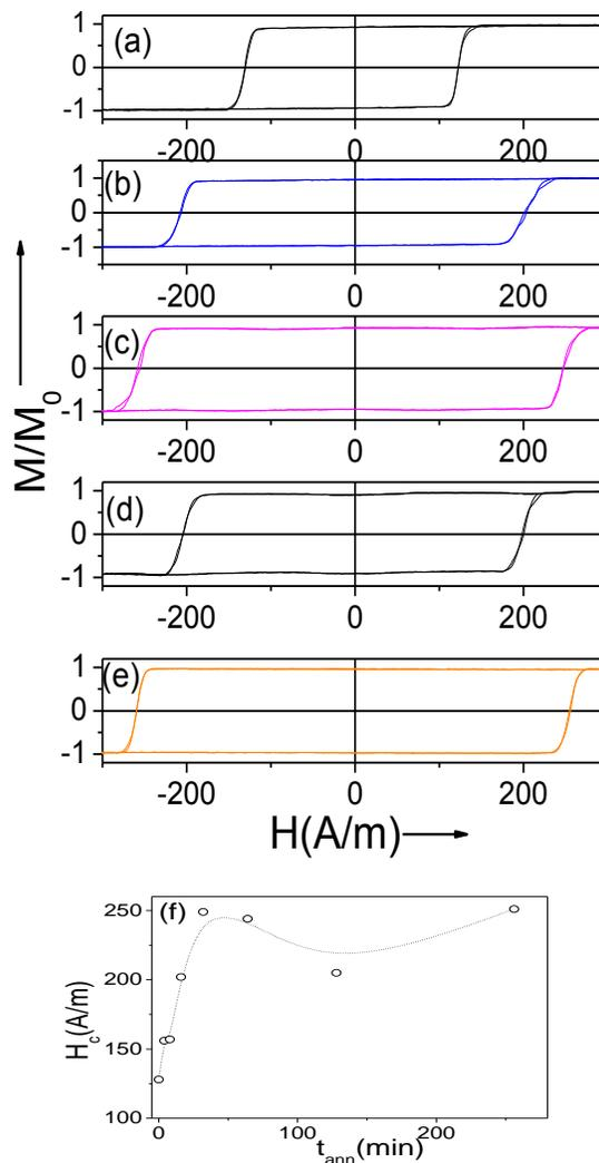
Figure 5. Hysteresis loops of as-prepared (a) and annealed at  $T_{ann} = 410$  °C for 16 min (b) 32 min (c), 128 min (d), and 256 min (e)  $Fe_{62}Ni_{15.5}Si_{7.5}B_{15}$  microwires and  $H_c(t_{ann})$  dependence of the same microwire.
