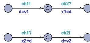
Figure 4. A native UPPAAL model for an exchanger
