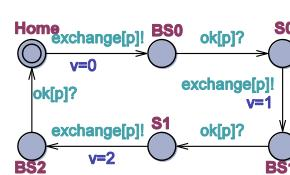
Figure 7. Producer automaton
