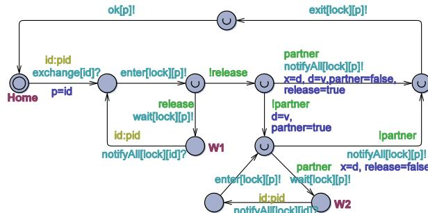
Figure 6. The Exchanger automaton based on JMonitor
