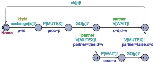
Figure 12. The ExchangerS automaton based on semaphores
