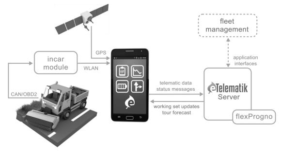
Figure 1. eTelematik system architectur overview (adapted figure, based on original by Johannes Kretzschmar, University Jena)
