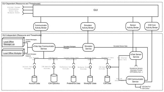
Figure 2. eTelematik mobile client's internal module overview
