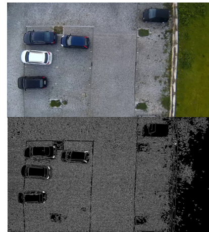
Figure 12. At the top, an image of a Block Pavement Parking. On the bottom the corresponding gradient Image.
