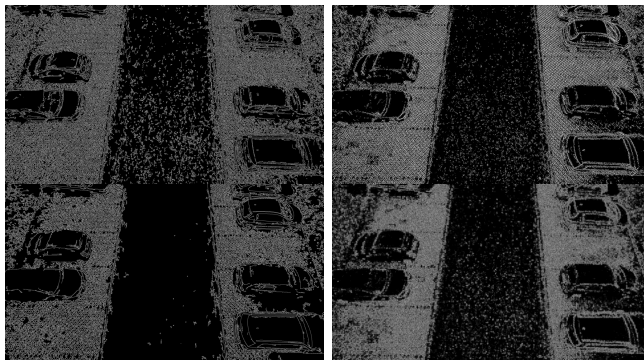
Figure 27. Two different edge detection algorithms tested with different parameters. From left to right, top to bottom: Canny Min=10, Max=50, Sobel X=1, Y=1, Canny Min=2, Max=200, Sobel X=2, Y=2.
