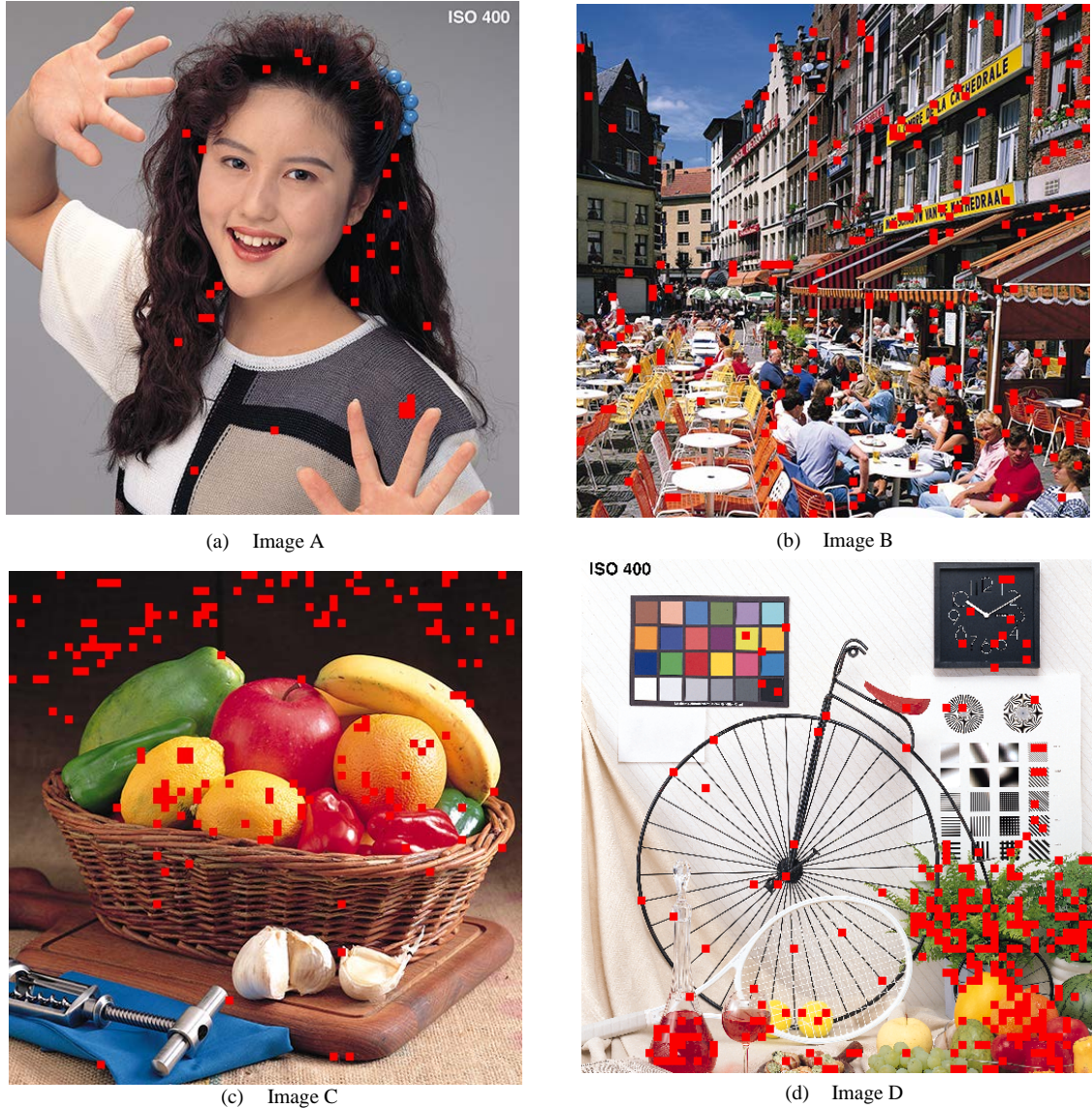
Figure 7. Blocks where readout error occurred when HC was set to one. Red squares indicate blocks where readout error occurred.
