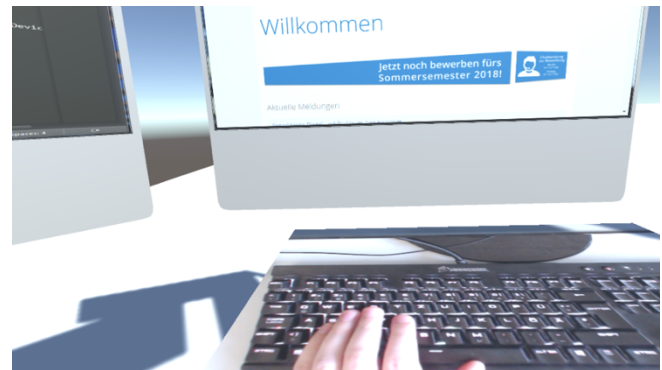
Figure 5. MR, showing real keyboard in cutout of VR desk and displays.
