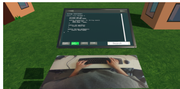
Figure 1. Coding with MR view of keyboard and mouse blended in and scroll bar shown on the virtual tablet.
