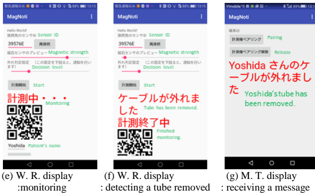
Figure 14. Drip monitoring system prototype.
