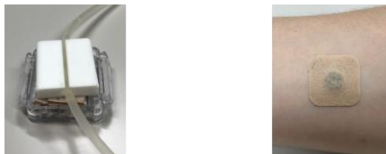
(a) Magnetic sensor and attached tube. (b) Magnetic patch on an arm.
