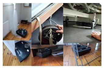
Figure 6. Situations where the robot got stuck and needed facilitation work
