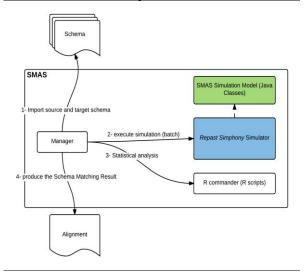
Figure 11. High-level Architecture for Reflex-SMAS
