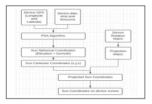
Figure 16. PSA algorithm integration in the application.
