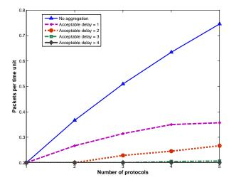
Figure 6. Required number of packets per time unit when using global aggregation with multiple protocols ( $\Delta T_i = i + 4$ ).
