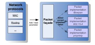
Figure 2. Through a packet façade, protocols interact with packets. Protocols do not require any knowledge about the actual packet construction.
