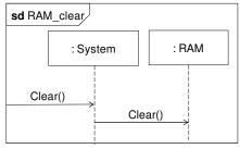
Figure 2. RAM clearing process.
