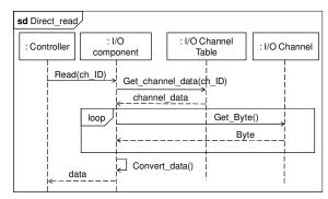
Figure 11. Process featuring direct access to I/O channels.
