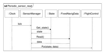
Figure 5. An elementary function triggered by the clock.
