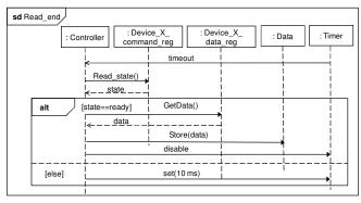
Figure 10. The timer triggers the conclusion of the operation.
