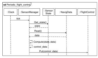
Figure 18. Sensor-driven flight control.
