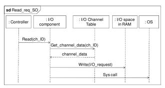
Figure 12. Process Access to I/O channels via the O.S.
