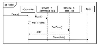
Figure 7. Device read specifications not mentioning time delay.
